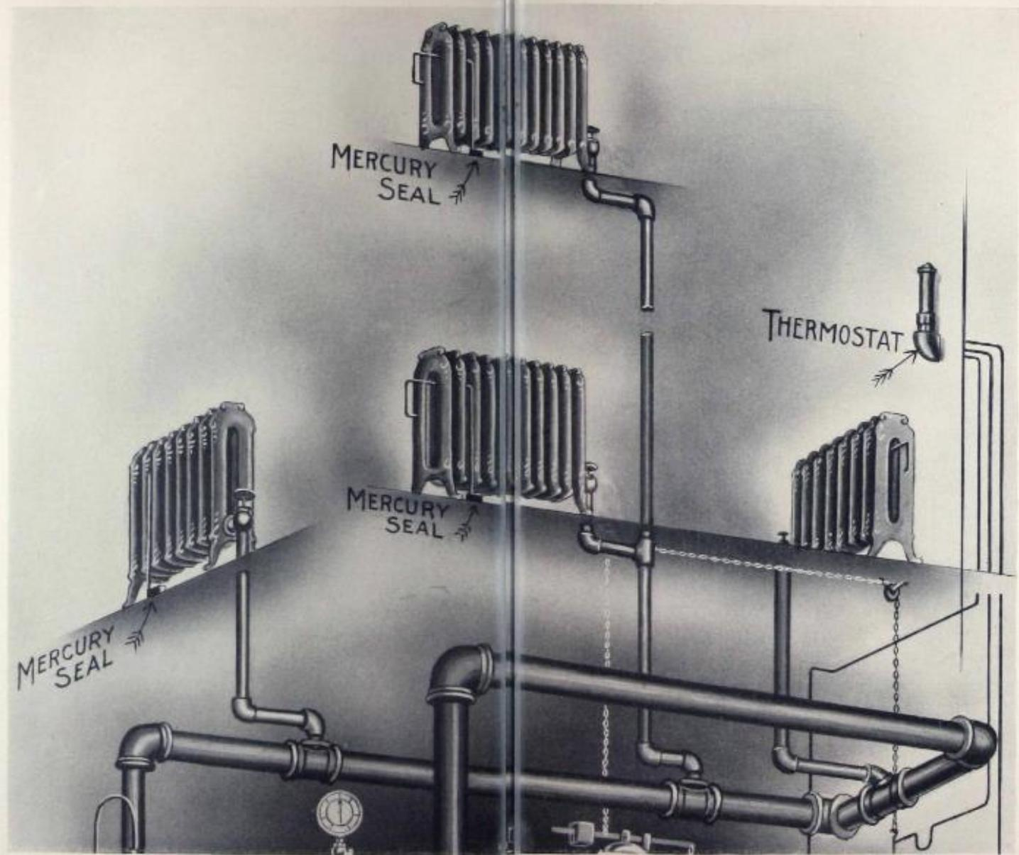
Plate VI gives a general illustration of the Direct Mercury Seal Vacuum Heating System. This plate is intended to be of sufficient size to enable the reader to thoroughly understand the construction and arrangement of the Jas. A. Trane Direct Mercury Seal Vacuum Heating System.
